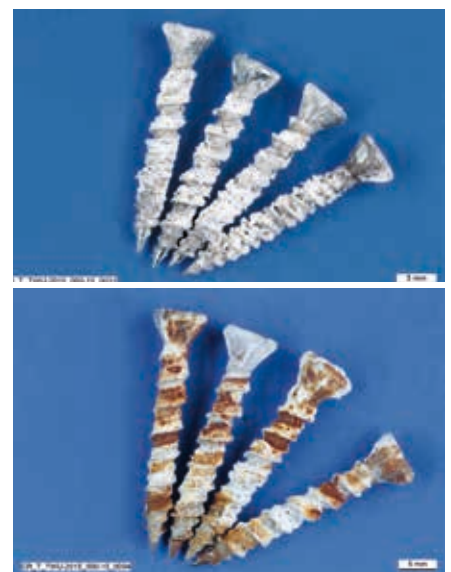
Fig. 14: Electrogalvanized screws with around 5 µm zinc coating after 48 h (up) and 96 h (down) in the salt spray test.
