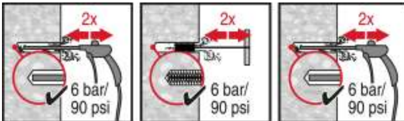
Compressed air cleaning (CAC)
