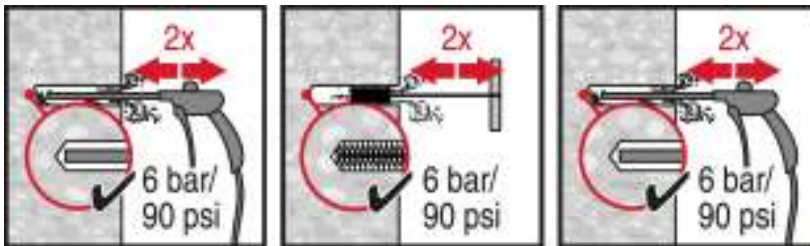
Compressed air cleaning (CAC)
