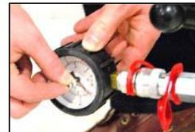
**4. Hold the HAT 30 by the grip while increasing the load on the HAP 1.15 by turning the crank in a clockwise direction. Increase the load until proof load of 26.5 kN is attained.**
