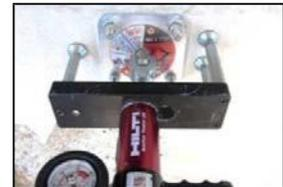
Turn crank in clockwise direction until legs are in contact with the base material.
