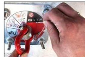
**8. Install the shackle and plug in the safety pin, optional is to mark or label the HAP 1.15 with date of proof loading, name of testing person**
