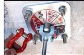
**2. Connect HAT 30 with ring bolt adapter and position the tester with edges of tester baseplate parallel to edges of HAP plate.**
