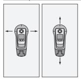
In order to achieve best results, the tool should be used with a sweeping motion (extended horizontal and vertical movements over the object). The series of illustrations show the sweep method in use. When the tool is switched on for the first time, it displays an animated training program that shows how the tool should be used to scan a surface.
