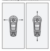
In order to achieve best results, the tool should be used with a sweeping motion (extended horizontal and vertical,
