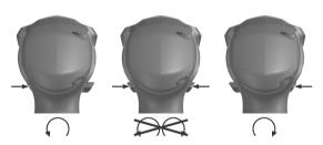
▶ Set the forward/reverse switch to the desired direction of rotation.
